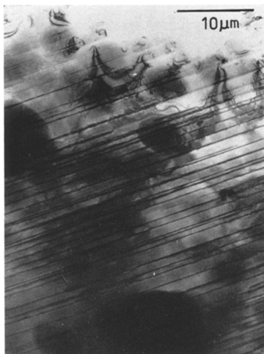
Figure 2 Low-magnification transmission electron micrograph (1000 kV) of grain in Fig. 1. The electron beam is approximately parallel to (100). The volume fraction of lamellae is obviously much lower than it appears to be in Fig. 1.
