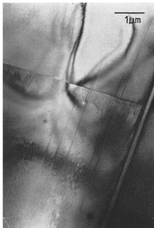
Figure 7 Bright-field electron micrograph (100 kV) showing heterogeneous nucleation of augite on a subgrain boundary. The "organ-pipe" distribution has been produced by autocatalytic nucleation of successive lamellae.
