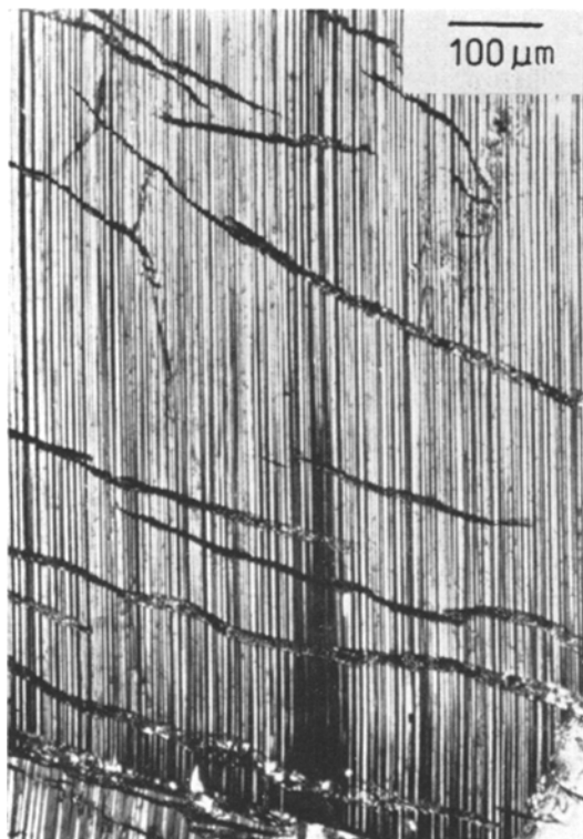
Figure 1 Optical micrograph of Stillwater bronzite (crossed polars) showing lamellar structure parallel to (100). Electron micrographs in Figs. 2 and 3 are from this area.
